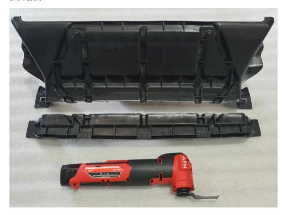
Once you have trimmed these parts replace them back on the vehicle and rivet the plastics back together again. Please note that rivets are not supplied with the fitting kit.
