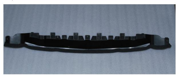
The next step is to remove the balance of the cooling deflectors. Please note that it is important to do this, and these plastics should not just be removed as part of the fitting process. You may choose to cut these without removing the rivets, but it may be difficult. For the purpose of this document, we have drilled out the 3 rivets each end so as to separate the pieces. This made it easier to trim the parts as required.
