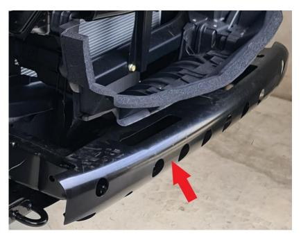
Remove the front Plastic deflector and discard. This part is held on with 2 rivets, one on each end and several plastic clip-in tabs.
