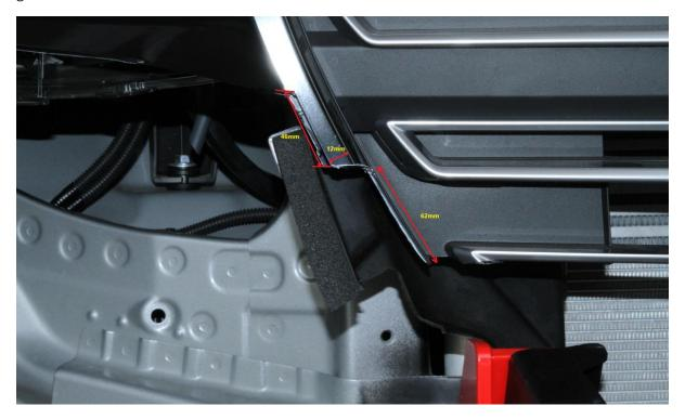
The eyelids need to be cut along the bottom edge. This is a continuation of the existing edge and should be marked using masking tape or similar. Extend the line from the corner on the outer edge of the headlight to the point where it makes joins the edge of the grille as highlighted below. Deburr all edges once cut.
