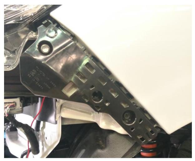
After Removal of the Fender Retaining clips there are 2 areas that need to be trimmed.
