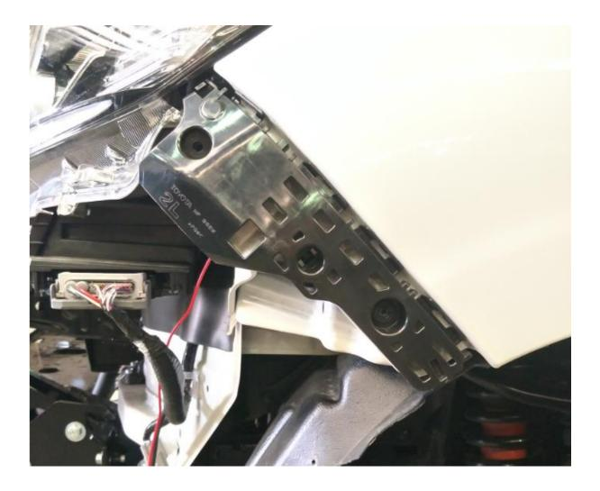
Once the retaining clips have been fitted then proceed to secure the new infill panel. Please note that the original OEM screws are used to secure this panel.
