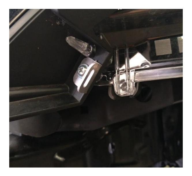
Trial Fit the panels under the Headlights. Please note that this panel may need to be trimmed once the Bullbar is fitted. It is recommended to fit this panel once the Bullbar alignment is correct.
