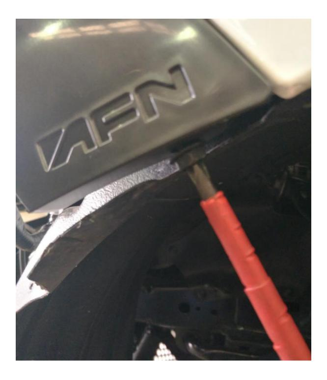
As per the image below fit the retaining clips that will secure the Headlight infill panel.
